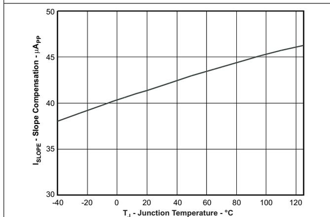
Figure 11. Current Slope Compensation Current vs Temperature
