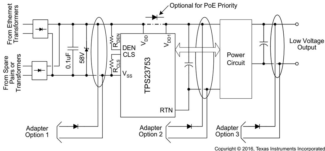
**Figure 22. ORing Configurations**
