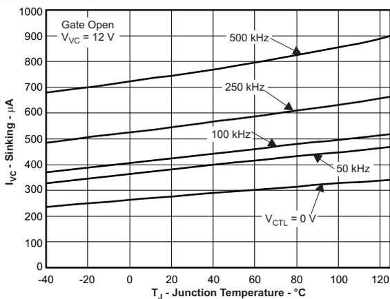
Figure 5. Controller Bias Current vs Temperature
