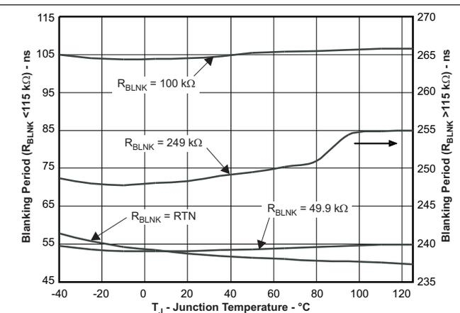
Figure 12. Blanking Period vs Temperature
