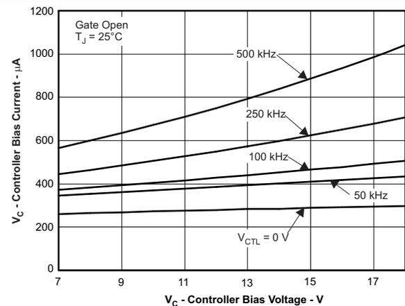
Figure 6. Controller Bias Current vs Voltage
