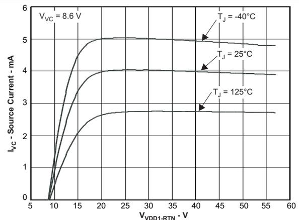
Figure 4. Converter Start-Up Source Current vs V\_VDD1
