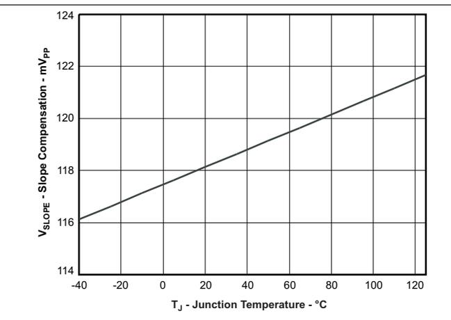
Figure 10. Current Slope Compensation Voltage vs Temperature
