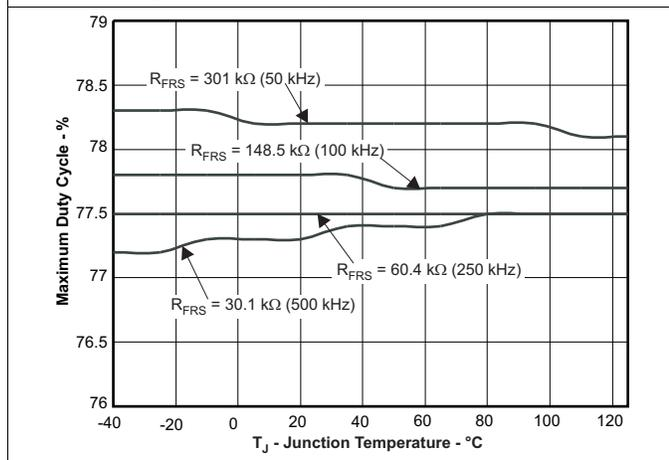
Figure 9. Maximum Duty Cycle vs Temperature
