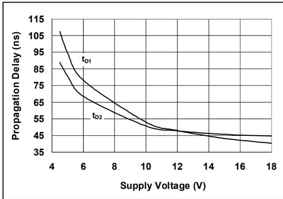
**FIGURE 2-7:** Propagation Delay Time vs. Supply Voltage.
