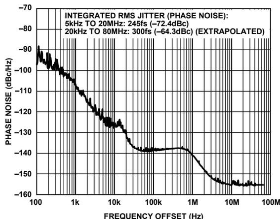
Figure 12. Absolute Phase Noise (Output Driver = LVPECL),  $f_R = 19.44$  MHz,  $f_O = 155.52$  MHz, LBW = 1 kHz,  $f_{SYS} = 50$  MHz (Crystal), PLL On with 2x Frequency Multiplier,  $I_{CP} = 375$   $\mu$ A, LF = External (350 kHz)
