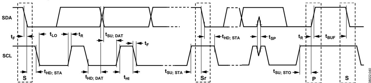
Figure 67. I<sup>2</sup>C Serial Port Timing
