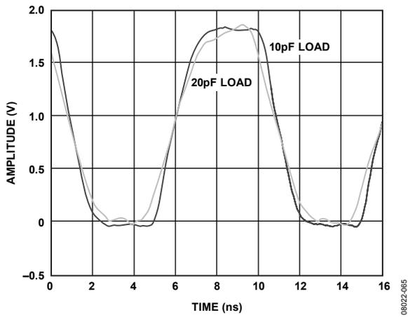
Figure 26. Output Waveform, 1.8 V CMOS (100 MHz)
