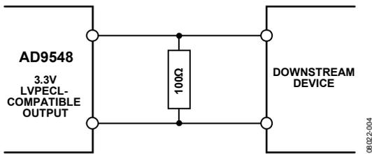
Figure 29. DC-Coupled LVDS or LVPECL Output Driver
