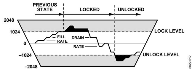
Figure 43. Lock Detector Diagram
