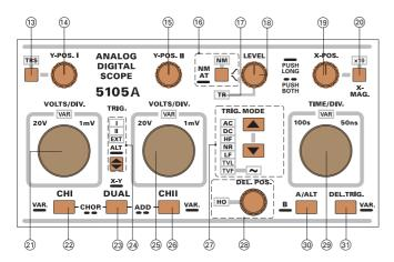
(27) TRIG. MODE - Pushbutton with double function and indicator LEDs.
