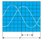
$t = \text{horizontal spacing of the zero transitions in div} \\ T = \text{horizontal spacing for one period in div}$
