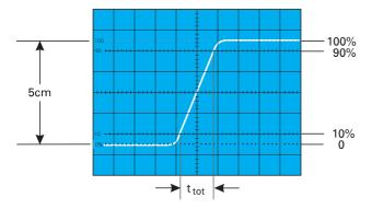
With a time coefficient of 5ns/div (X x10 magnification active), the example shown in the above figure results in a total measured rise time of
