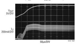
12V Boost Converter Start-Up without Input Current Limit ( $V_{IN}$  = 1.8V,  $I_{LOAD}$  = 40mA)
