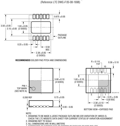
DD Package 10-Lead Plastic DFN ( $3mm \times 3mm$ )
