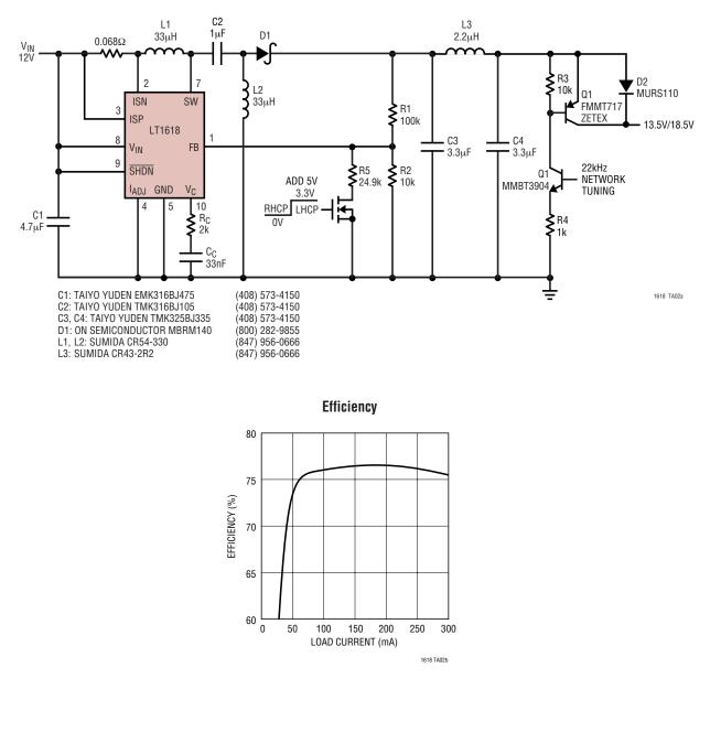
4.5W Direct Broadcast Satellite (DBS) Power Supply with Short-Circuit Protection
