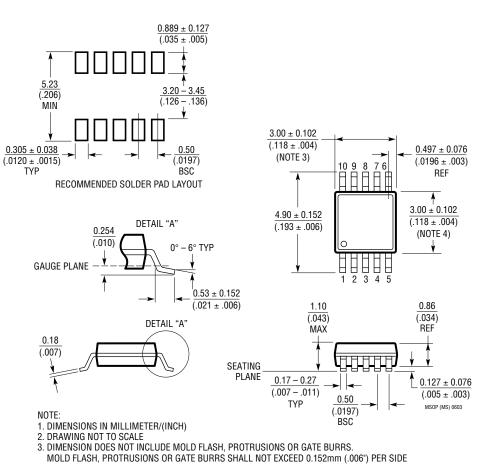
**MS Package 10-Lead Plastic MSOP** (Reference LTC DWG # 05-08-1661)
